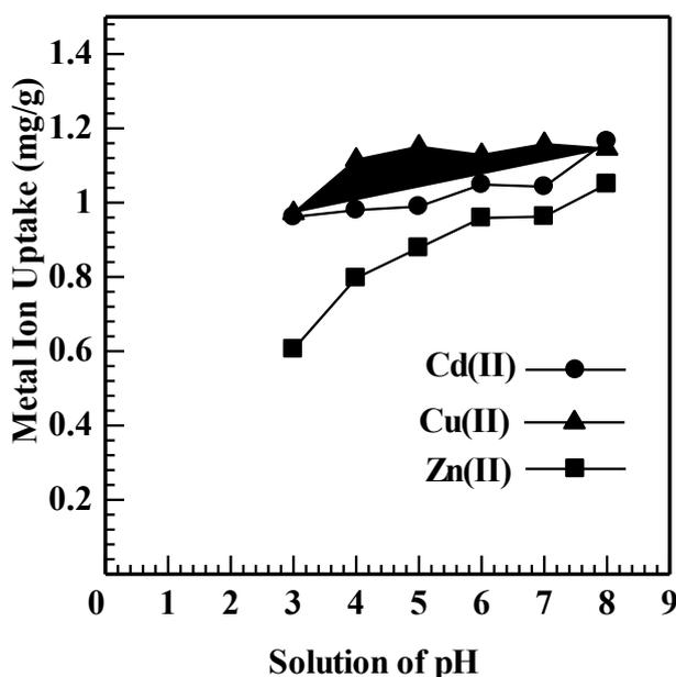
Figure 2. Effect of pH Solution on the metals ion removal by Salak Seeds.
