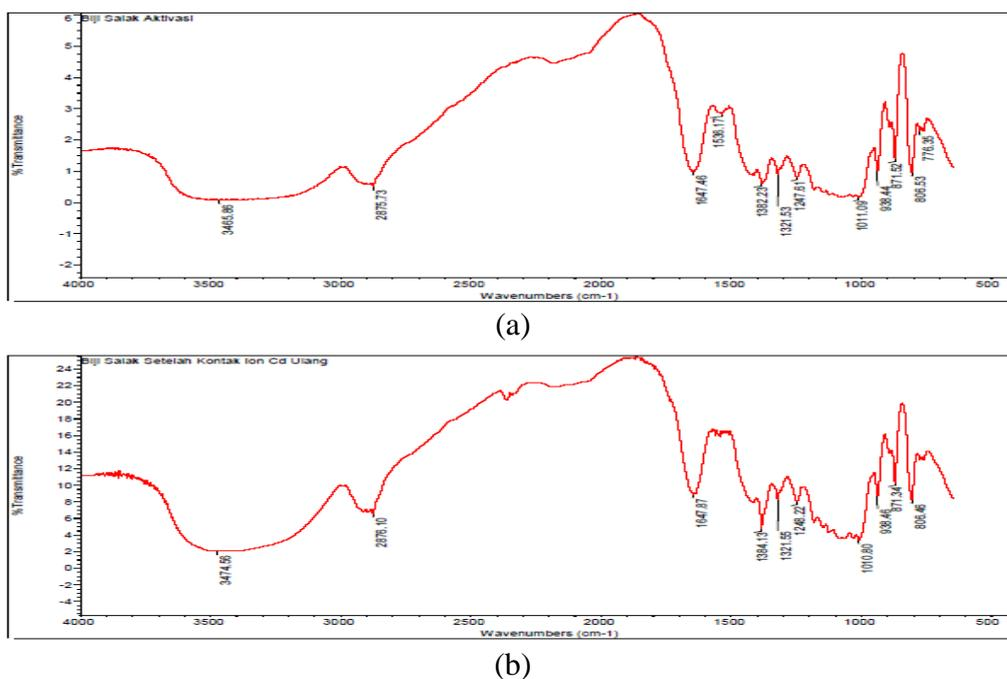
Figure 1. FT-IR spectrum of salak sheed before (a) and after (b) removal of Cu(II) ions.
