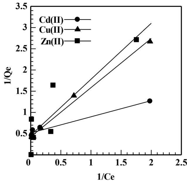
Figure 5. Isotherm Langmuir of Cd(II), Cu(II) and Zn(II) ion removal by Salak Seeds.
