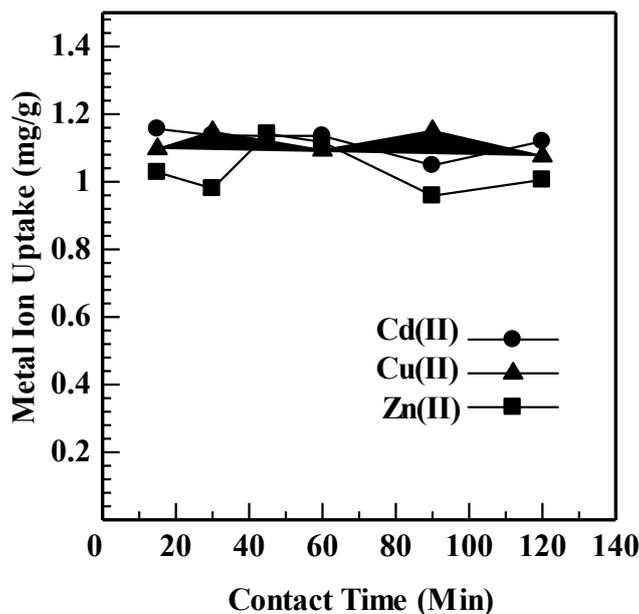
Figure 3. Effect of contacting time on the Cu(II), Cd(II) and Zn(II) removal by Salak Seeds.
